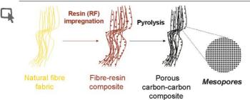
Porous carbon-carbon composite replicated from a natural fibre
